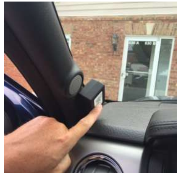
6. Unit mounted on A-pillar using provided 3M tape with ODB extension cable tucked behind dashboard
