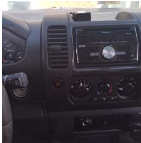
5. Unit mounted above radio with ODB extension cable tucked behind dashboard
