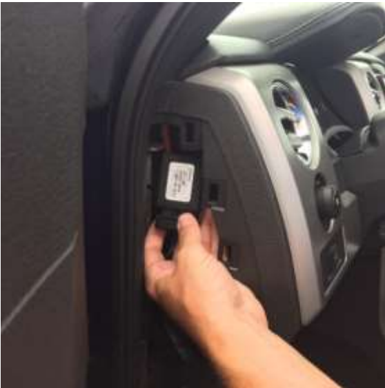
4. Unit with ODB extension cable tucked completely behind the dashboard
